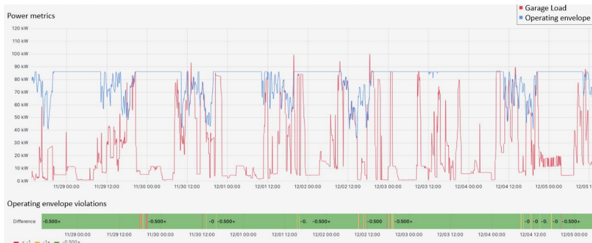
Figure 2: Overview of grid restriction violations based on measured data on charging power of electric vehicles for dynamic charging power limitation.
